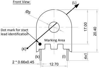
All dimensions are in mm Linear dimensional tolerance ±0.2mm
